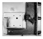
1. The mounting surface for the lock should be smooth and flat, with 1/4-20 (or M6) mounting screw holes. The wire channel (spindle hole) must have a minimum diameter of 5/16 inch (8 mm). Use a reamer or file to remove any sharp edges from the wire channel (spindle hole) that might damage the wire cables. Do this on the inside and outside of the safe door.
